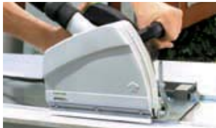
A closed extraction hood and sealing brush for maximum dust extraction.
